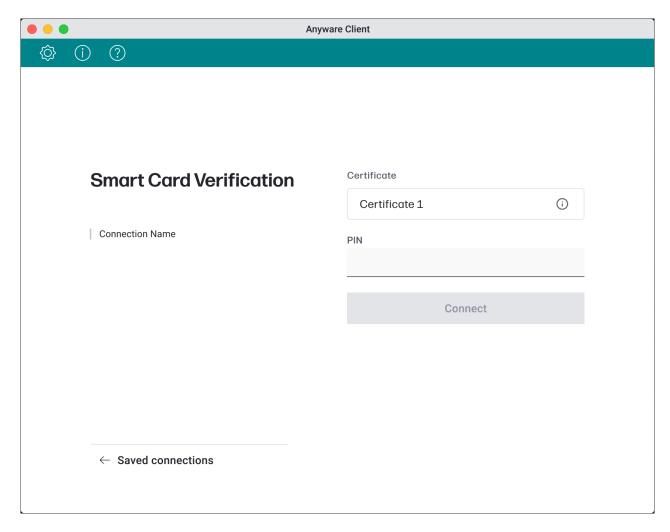
• If the client detects **multiple certificates**, on the **Smart Card Verification** window, select a certificate, provide the smart card PIN, and click **Connect**.
